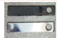
Pristine and oxidized Stainless Steel (316-1.4571)
