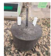
Corrosion tests in mortar under saturated conditions
